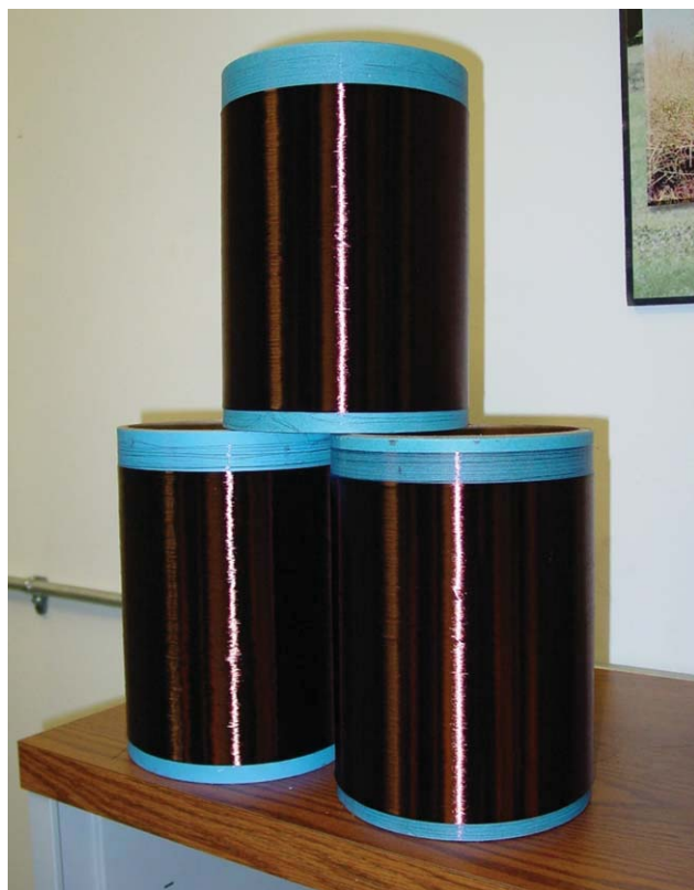
Figure 3 Spools of fibers produced from HWL-OP lignin utilizing the pilot scale unit with 12-hole spinneret. [Color figure can be viewed in the online issue, which is available at wileyonlinelibrary.com .]
